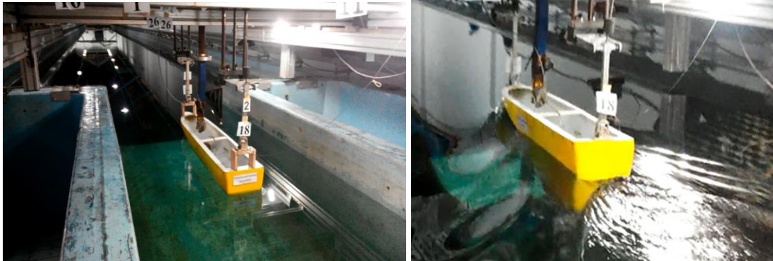
Figure 2. Resistance test at ITS Hydrodynamic Laboratory
